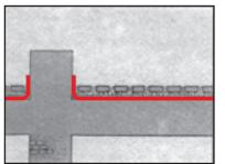
other suitable protection layer over the waterproofing membrane followed by insulation boards (If required) and place the topping screed of 4 cm to 5 cm thickness or suitable cement tiles.
