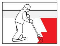
each coat, two different colours of ROOFGUARD should be used.
