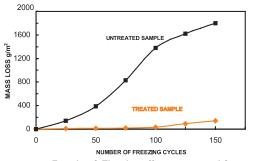
Freezing & Thawing effects on treated & untreated concrete samples
